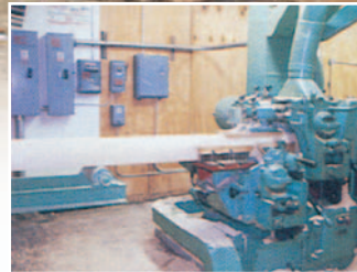
Custom machining the cant into the double tongue-and-groove log wall component.
